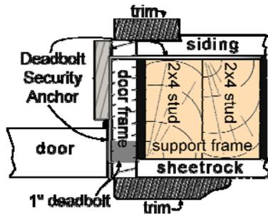
Using 16 gauge cold rolled steel this industrial strength strike plate uses both 2x4s to anchor the faceplate onto the door frame. Break-ins would require either both 2x4s to break or tear the plate's 9000 psi rating. With its unique adjustable replacement cleat design the Deadbolt Security Anchor is quick and easy to install and does not require adjustments of the door or door frame. It is visible from the exterior acting as a deterrent.
