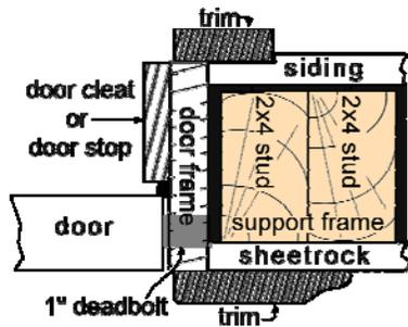
Most door hinges and strike plates are only attached to 1/2" thick, soft wood door trim using small, short, weak 1/2 inch brass screws. As you can see in the illustration above, most doors are not truly even attached to the wall itself (the 2 x 4 studs), but only to the soft wood trim. The air space is there to allow 'squaring' of the door frame so the door will hang level, open, and close properly.
